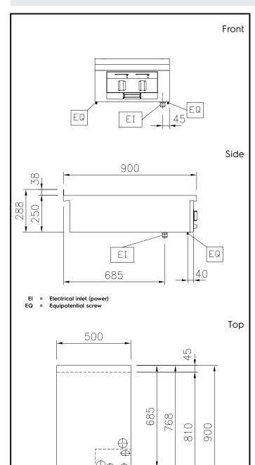
**Electric** Supply voltage: 400 V/3N ph/50/60 Hz Total Watts: 6 kW **Key Information: Working Temperature MIN:** 100 °C **Working Temperature MAX:** 450 °C 500 mm External dimensions, Width: External dimensions, Depth: 900 mm External dimensions, Height: 250 mm Net weight: 75 kg Configuration: One-Side Operated;Top Front Plates Power: 3 - 0 kW **Back Plates Power:** 3 - kW Solid top usable surface 360 mm (width): Solid top usable surface 730 mm
